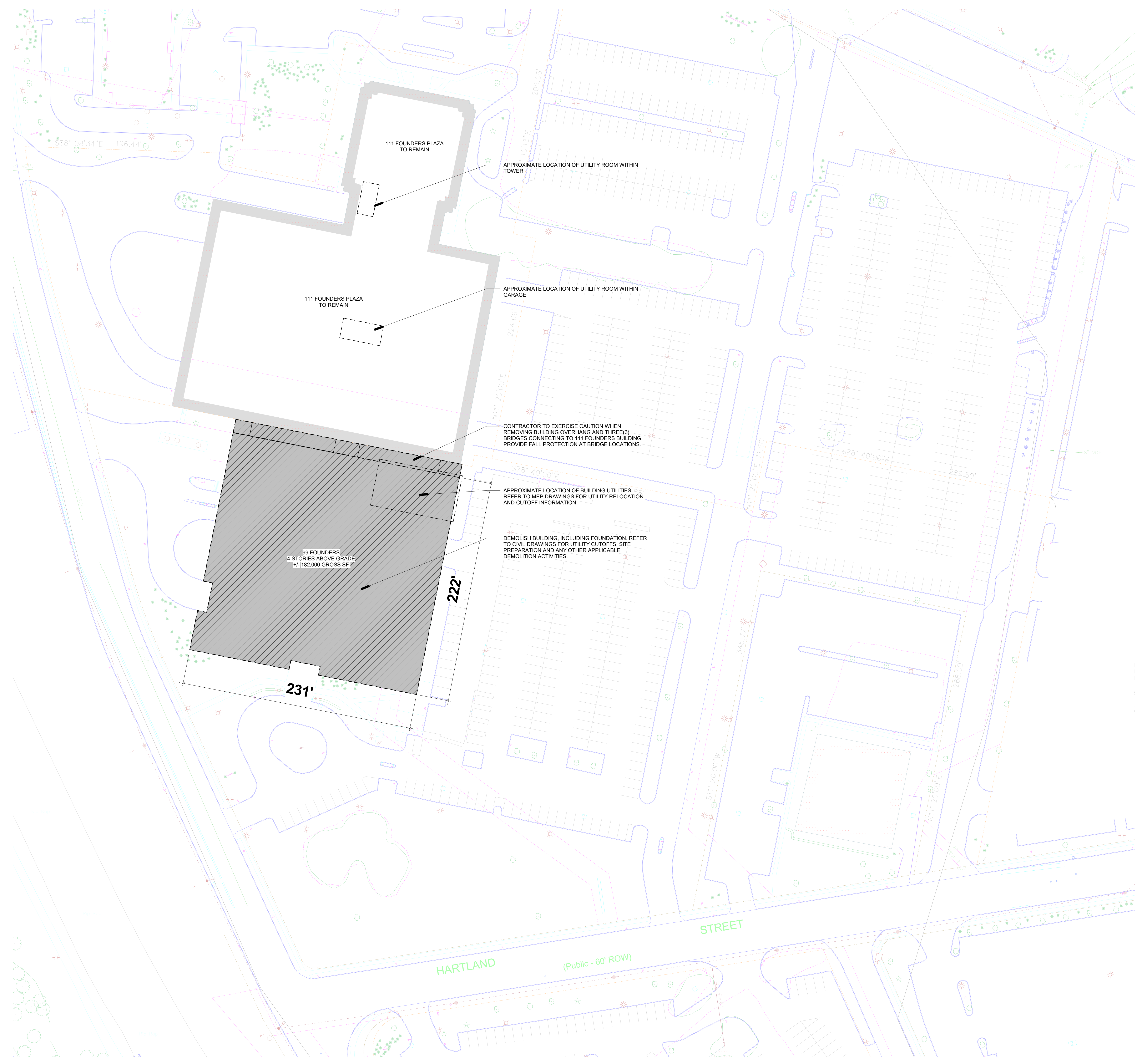
1 99 FOUNDERS DEMOLITION PLAN SCALE: 1" = 40'-0"
