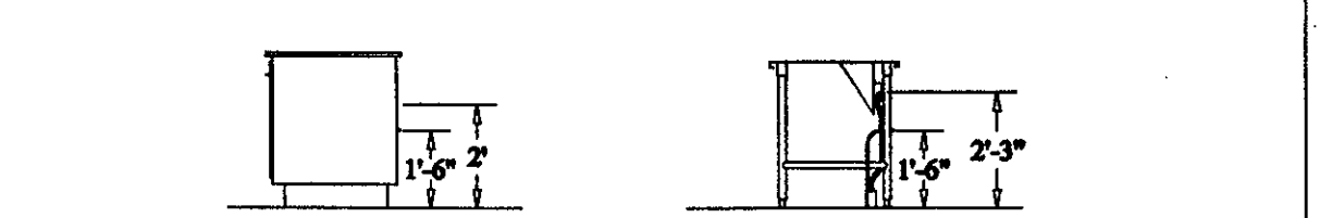
TYPICAL ELECTRICAL AND PLUMBING CONNECTIONS FOR ISLAND REAR COUNTERS, MILLWORK AND STAINLESS STEEL
